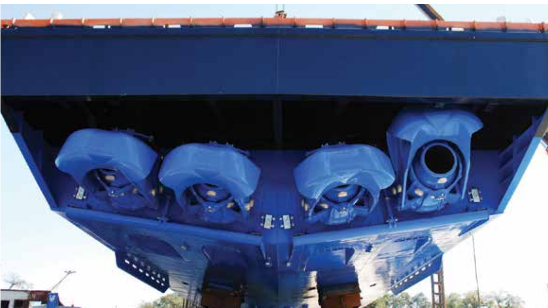
Above and Below: Crewboat "Aaron McCall" was the first vessel to be fitted with quadruple HamiltonJet HT900 waterjets
